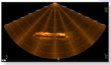
900kHz image of German Schnellboot(fast boat), these craft were 35m long and 5.1m in beam. Data collected with M900/2250-130/45 which shares similar array configuration for 900kHz.
